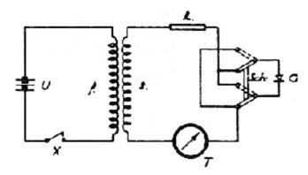
On the secondary side the coils S was connected with resistance R, a reversible rectifier G, and a highly sensitive hot-wire ammeter, form a circuit. The resistance R was large compared with the apparent resistance of the coils S.
