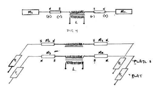
This device consists of an arrangement of magnets, flat coils, and copper plates, with a primary circuit energized by a small dry battery. The output from the secondary was used to light a bank of lamps and was claimed to be many time the original input, and to continue indefinitely. Details of this circuit, and a theory as to its mode of operation were given (summarized in Appendix I).
